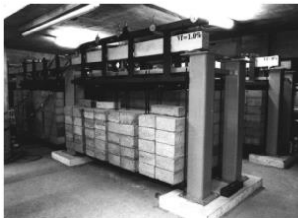
Fig. 1 Experimental Setup For Testing Frc Beams (Authorized Reprint From)
